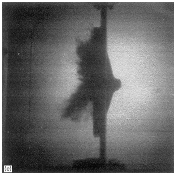
Figure 3 A series of high-speed photographs of alumina/FRP (B type) target material with an adhesive layer thickness of 2.3 mm: the projectile-striking velocity was 729 \text{ m s}^{-1} (a) 0 \mu\text{s} , (b) 28.6 \mu\text{s} , (c) 57.2 \mu\text{s} , (d) 85.8 \mu\text{s} , (e) 114.4 \mu\text{s} , (f) 143.0 \mu\text{s} , (g) 171.6 \mu\text{s} , (h) 200.2 \mu\text{s} , (i) 228.8 \mu\text{s} , (j) 257.4 \mu\text{s} , (k) 286.0 \mu\text{s} , (l) 314.6 \mu\text{s} .
