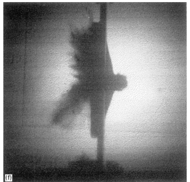
Figure 3 A series of high-speed photographs of alumina/FRP (B type) target material with an adhesive layer thickness of 2.3 mm: the projectile-striking velocity was 729 \text{ m s}^{-1} (a) 0 \mu\text{s} , (b) 28.6 \mu\text{s} , (c) 57.2 \mu\text{s} , (d) 85.8 \mu\text{s} , (e) 114.4 \mu\text{s} , (f) 143.0 \mu\text{s} , (g) 171.6 \mu\text{s} , (h) 200.2 \mu\text{s} , (i) 228.8 \mu\text{s} , (j) 257.4 \mu\text{s} , (k) 286.0 \mu\text{s} , (l) 314.6 \mu\text{s} .
