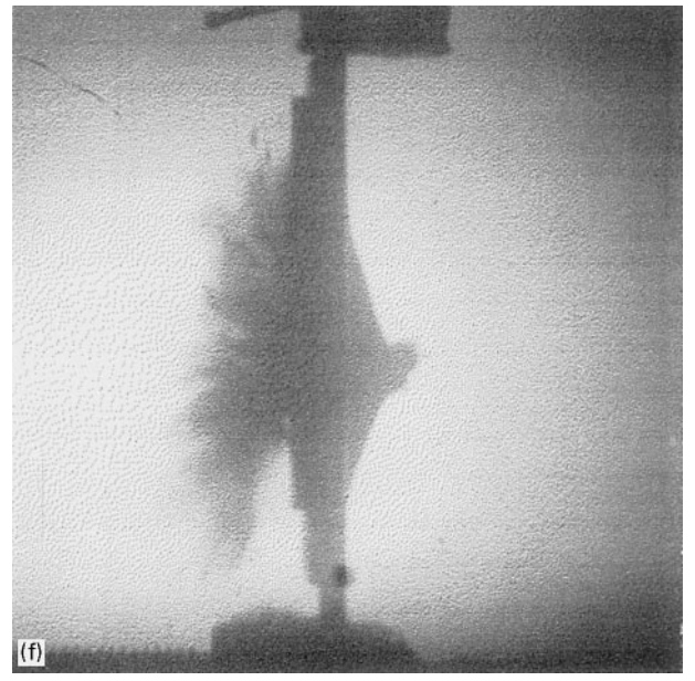
Figure 6 A series of high-speed photographs of alumina/FRP (A type) target material with an adhesive layer thickness of 2.3 mm: the projectile-striking velocity was 725 \text{ m s}^{-1} (a) 0 \mu\text{s} , (b) 28.6 \mu\text{s} , (c) 57.2 \mu\text{s} , (d) 85.8 \mu\text{s} , (e) 114.4 \mu\text{s} , (f) 143.0 \mu\text{s} , (g) 171.6 \mu\text{s} , (h) 200.2 \mu\text{s} , (i) 228.8 \mu\text{s} , (j) 257.4 \mu\text{s} , (k) 286.0 \mu\text{s} , (l) 314.6 \mu\text{s} .
